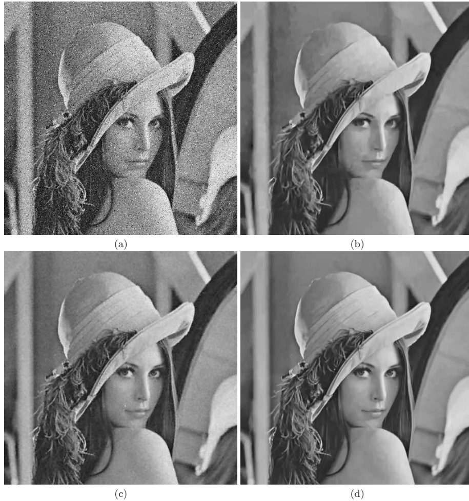
Fig. 5: (a) The Lena image corrupted by 20 dB of Gaussian noise and 10% outliers. (b) Denoising with BM3D (30.66 dB). (c) Denoising with KGARD (31.94 dB). (d) Denoising with joint KGARD-BM3D (33.81 dB).
